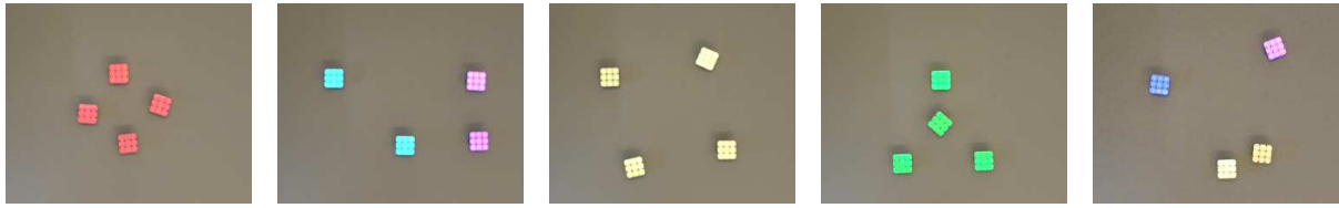
Fig. 5. Five patterns represented with only four robots. Left to right: circle, two lines, ring, triangle, three stars. Even with very low resolution patterns are noticeable
